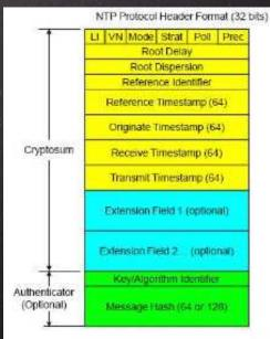
Authenticator uses DES-CBC or MD5 cryptosum of NTP header plus extension fields (NTPv4)
